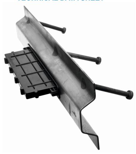
Conecto Omega 03NB is used as a day off work for the construction teams. The shape and dowel system prevent the least amount of vertical movement and guarantee optimal load transfers. Pulling rods guarantee solid anchorage in the concrete when shrinking occurs due to drying of the concrete, which also causes the actual widening to occur. The milled upper side ensures perfect smoothness of the 2 steel plates and lasting edge protection of the newly created floor.
