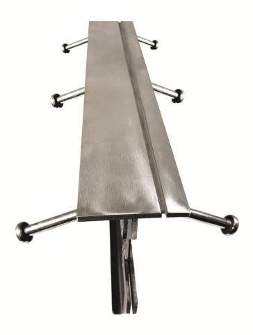
Conecto Sinus 06NE90 heavy-duty expansion joint profile is an essential solution for protecting and reinforcing joints in highly stressed concrete floors. This solution helps to clean top opening easier and faster. Additionally, it serves as permanent formwork for concrete floor, offering robust edge protection and effective load transfer through integrated dowel plates. Ideal for demanding applications, this profile guarantees durability and seamless performance.
