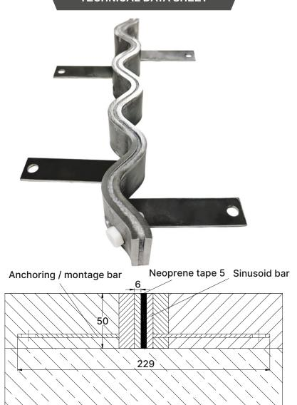
Conecto Sinus are reparation joints designed for cracking floors. Sinusoid construction provides two-level movement which prevent deeper cracking of the floors. Properly installed Conecto Sinus joints eliminate resultant damages and prevent in case of further damages. Properly secured with Conecto Sinus joints floor will not cause vehicles damages and ward off deep cracks which could prevent further usage of floor. Standard lenght = 2.4 meters.
