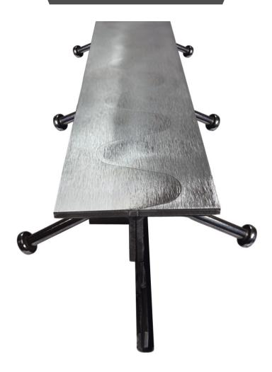
Conecto Sinus 06NC115 is heavy-duty joint profile for protecting and reinforcing joints in highly stressed concrete floors. Designed with a sinus wave, it ensures smooth, vibration-free travel for industrial forklift, regardless of tire size or hardness wheels. This innovative design minimizes noise and vibration and guarantees durability floor. It serves also as permanent formwork for concrete floors, offering robust edge protection and effective load transfer.
