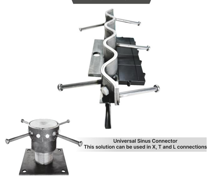
Conecto Sinus 4+4 is durable joint system featuring wave steel top that provide exceptional protection for slab edges. It effectively transfers horizontal loads between adjacent slabs, minimizing vertical displacement. The system enables smooth movement of forklifts and other vehicles, eliminating impact and vibrations. Sinus solution ensures a comfortable experience for forklift operators. Ideal for high-traffic areas, this solution combines strength, reliability, and ease of applications.
