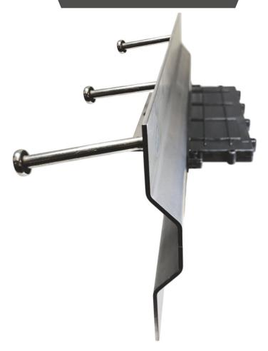
Conecto Omega 03NB is used as a day off work for the construction teams. The shape and dowel system prevent the least amount of vertical movement and guarantee optimal load transfers. Pulling rods guarantee solid anchorage in the concrete when shrinking occurs due to drying of the concrete, which also causes the actual widening to occur. The milled upper side ensures perfect smoothness of the 2 steel plates and lasting edge protection of the newly created floor.
